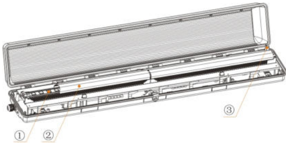
全塑防爆LED条形灯 CZ0866/2 × LED 30W□ Full plastic explosion-proof LED linear light fittings
